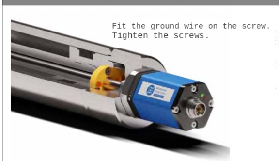
Base unit replacement (e.g. MSI-H sensor), part 2: 3 — insert the new base unit, fit the ground wire on the screw, tighten the screws
